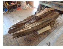
water. I soaked the wood with polyester resin thinned 100% with acetone; after curing it was solid and could be handled without falling apart.
